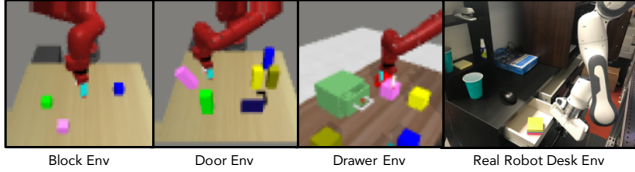
Figure 3: Experimental Domains. We consider 3 simulated domains, interacting with blocks, a door, and a drawer. We also test on a real Franka robot interacting with a desk.
